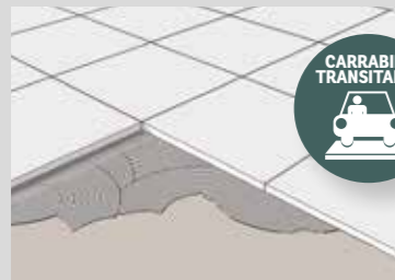
POSA SU MASSETTO CON COLLA Fuga consigliata di 5 mm INSTALLATION ON A SCREED WITH ADHESIVE Joint between tiles 5 mm
